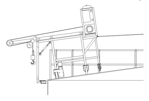
4. Lower or higher the SIDE SUPPORT ARM Wheels to avoid obstacles on the Tank Wall. If there are no obstacles, the ideal position is approximately 30 cm below the edge of the tank roof.
