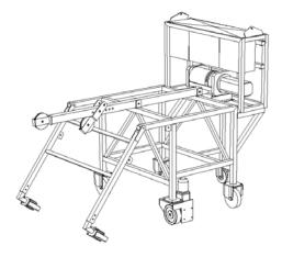
5. Attach TURN-BUCKLES to DRIVE FRAME and SIDE SUPPORT ARM.
