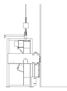
WARNING : When the machine is hoisted for the first time, hoist it only <u>10 cm</u> and check if all connections are fixed properly and make sure that the Safety Line on the tank roof is checked!
