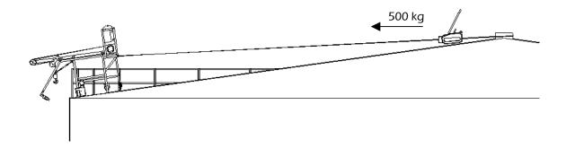
2. Pull the RIGGING SYSTEM with the Tirfor until the distance between the WINCH CABLE and the Tank Wall is 375 mm (if necessary move the PULLEY FRAME).
